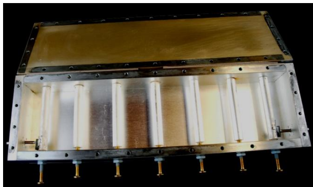
Figure 4 – Inside a cavity filter
