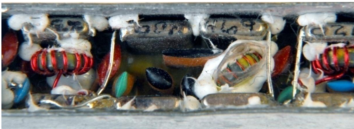
Figure 8 – Inside a crystal filter
